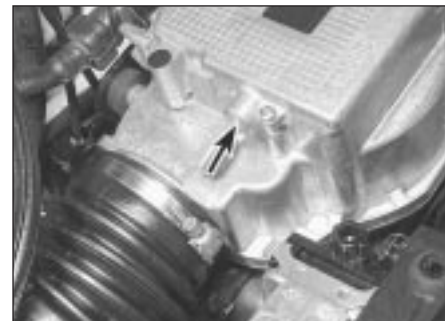
9.3 Mixture adjustment screw (arrowed)
