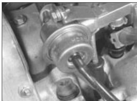
12.4b Pressure regulator attached to fuel rail
