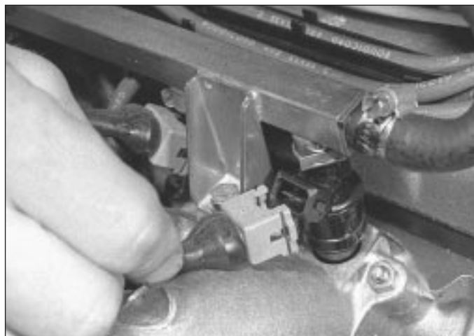
12.2 Disconnecting a fuel injector wiring connector
