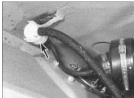
8.3 Vent valve location (arrowed) - GTi
