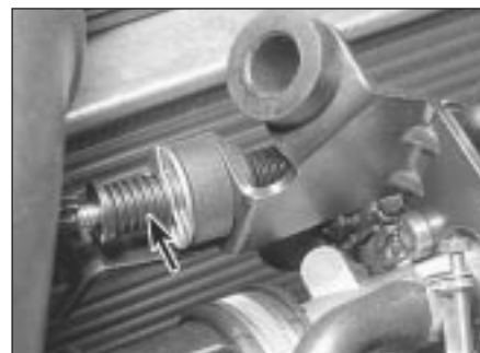
13.1 Accelerator cable adjustment ferrule (arrowed)
