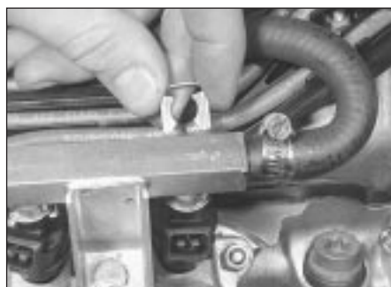
12.3b Fuel rail/injector clip
