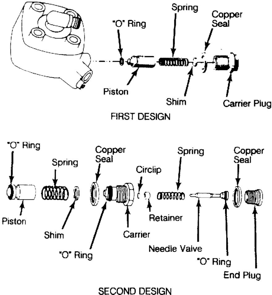
Fig. 10: Pressure Regulator in Fuel Distributor
