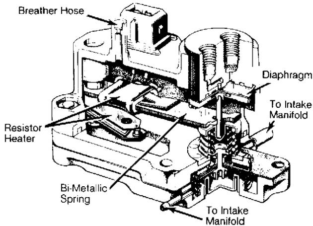
Fig. 2: Control Pressure Regulator
