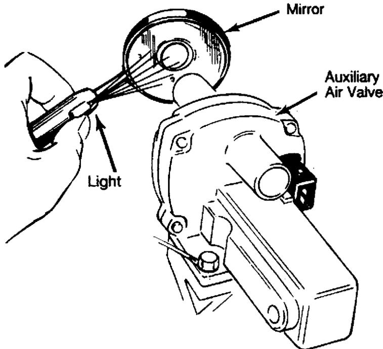
Fig. 12: Checking Auxiliary Air Valve Operation
