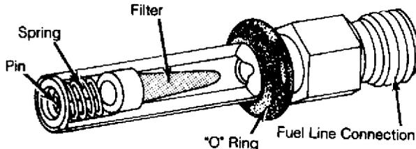
Fig. 3: Bosch CIS Lambda Injection Nozzle
