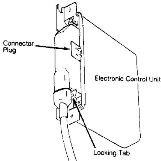
Fig. 4: Bosch CIS Lambda Electronic Control Unit
